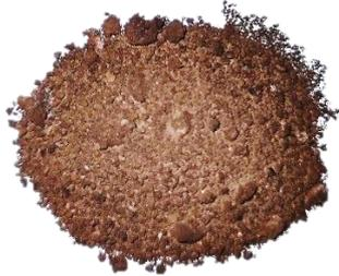
Gambar III.8 Frit Hasil Fusi Alkali
