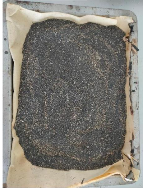
Gambar A.2 Sampel Pasir Ilmenit
