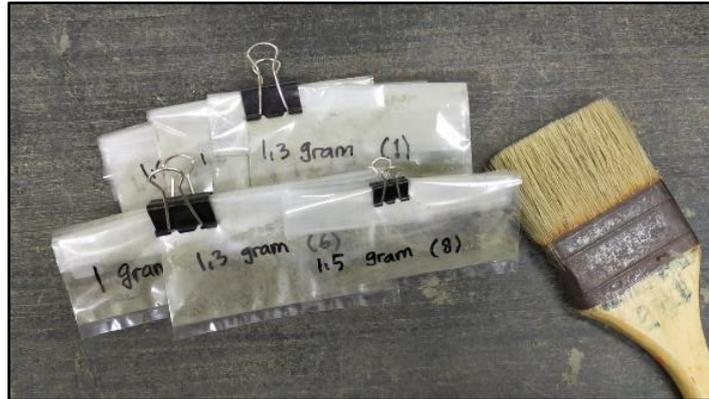
**Gambar 5.** Sampel ukuran 200 mesh (*powder*)
