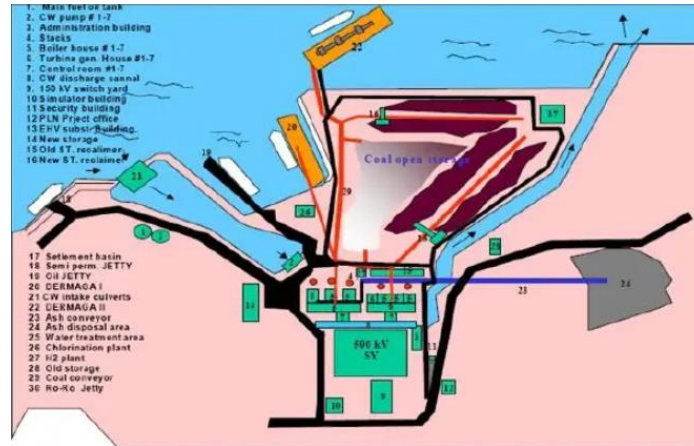
Gambar I.1.2.2.2. Layout PT PLN Indonesia Power UBP Suralaya (Sumber: PT Indonesia Power Suralaya)
