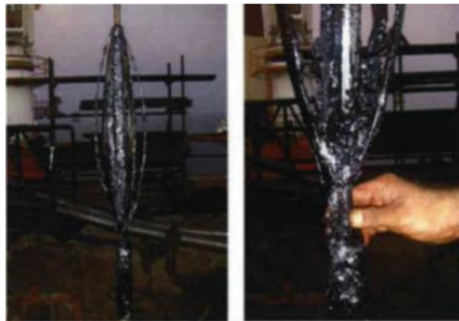
Figure 5. Scale Deposition on Cutter Gauge Slickline at HPS Field
