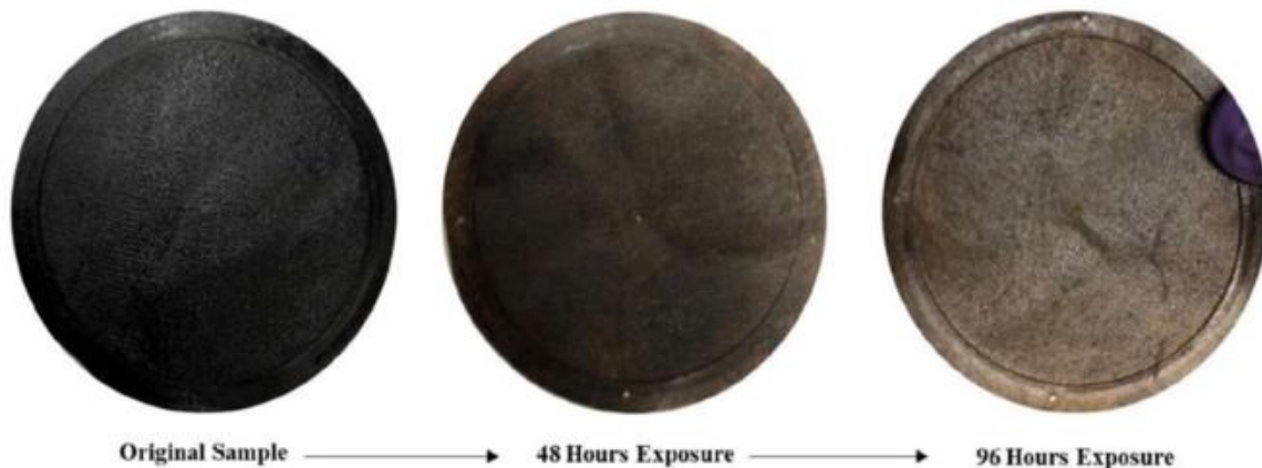
Figure 8. Evaluation of Asphaltene Content in HPS Field Oil Samples after the Squeeze Asphaltene Inhibitor Program
