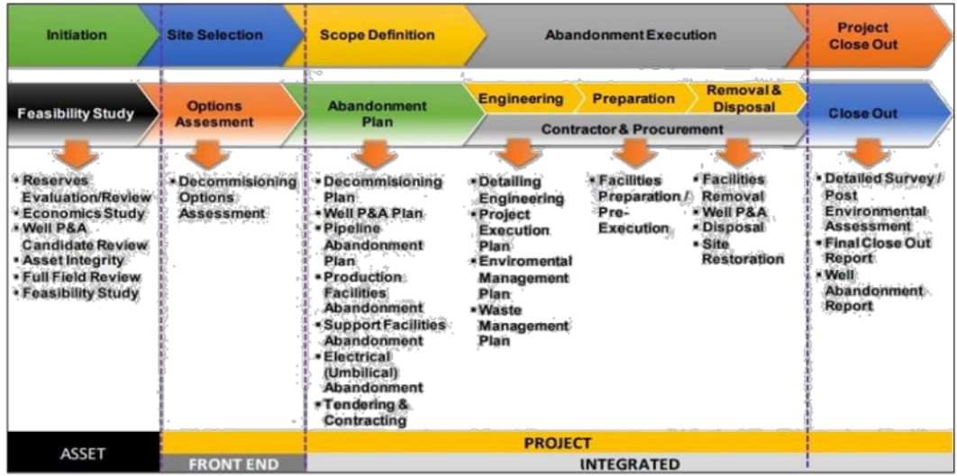
Fig. 4. Road Map for Oil Production Platform Decommissioning
