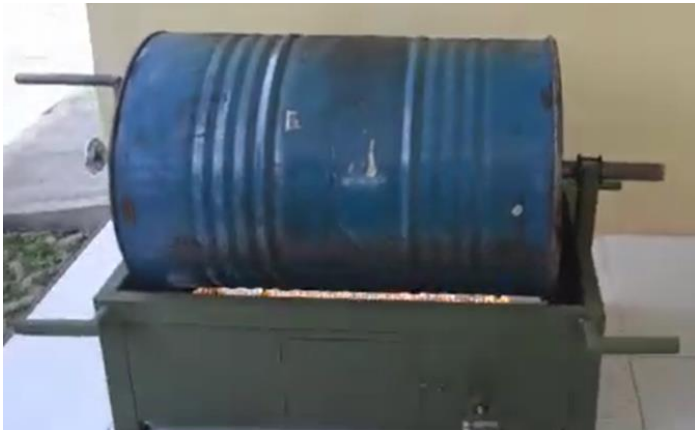
Gambar 8 Tabung Pembakaran Rotary Drum Pyrolizer (RDP)
