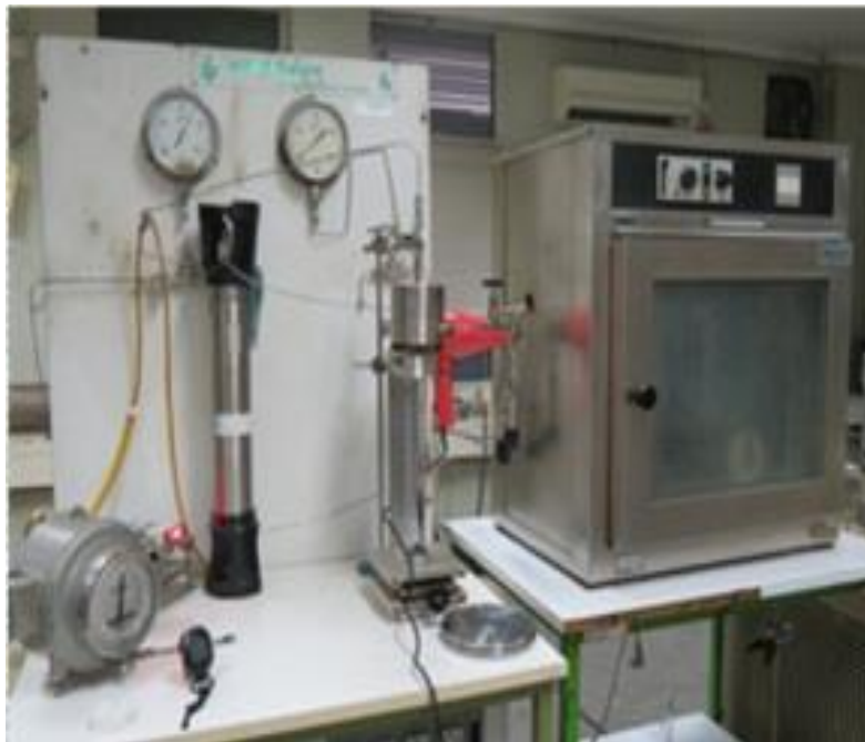
Figure 3: MMP determination apparatus in the laboratory using slimtube.
