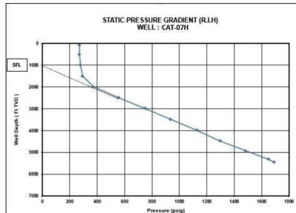
FIGURE 2. BHP Survey of CAT-07H
