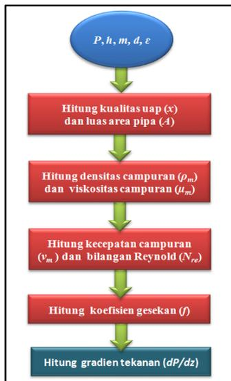
**Gambar 10. Prosedur Perhitungan Gradien Kehilangan Tekanan Model *Homogenous***
