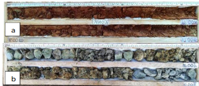
FIGURE 13. Saprolit ore zone (a) earty saprolit (b) rocky saprolit
