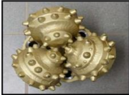
Gambar 4.2 Roller Tricone Bit
