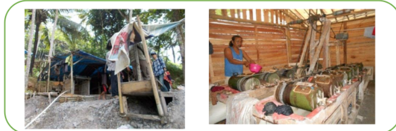
Figure 03. Condition of hole in local mining area and the drum to accommodate the gold ore.
