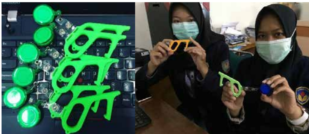
Gambar 5. Hasil 3D printing alat safety finger extension .
