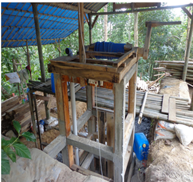
Fig.2. Vertical Tunnel (Shaft) at ASGM
