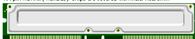
184-pin RDRAM (Rambus) Chips are covered with metal heat sink.
