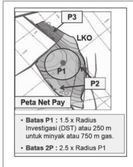
Fig 5. Distribution of Reserve Areas by Well Radius (Dadang Rukmana, Technical Aspect Subsurface, 2014)
