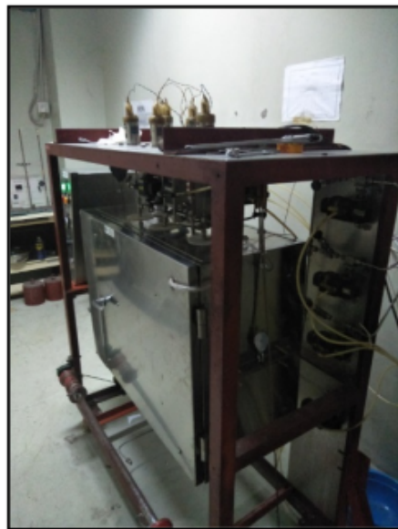
Gambar 14. Tabung Pressure Transmitter dan Oven Isotherm
