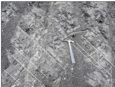
Fig 6. Cleat system of Seam A-1
