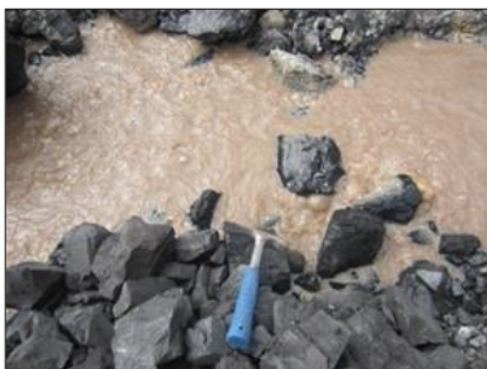
Fig. 7. The Gases bubble on permeability by cleat system of Seam A-1
