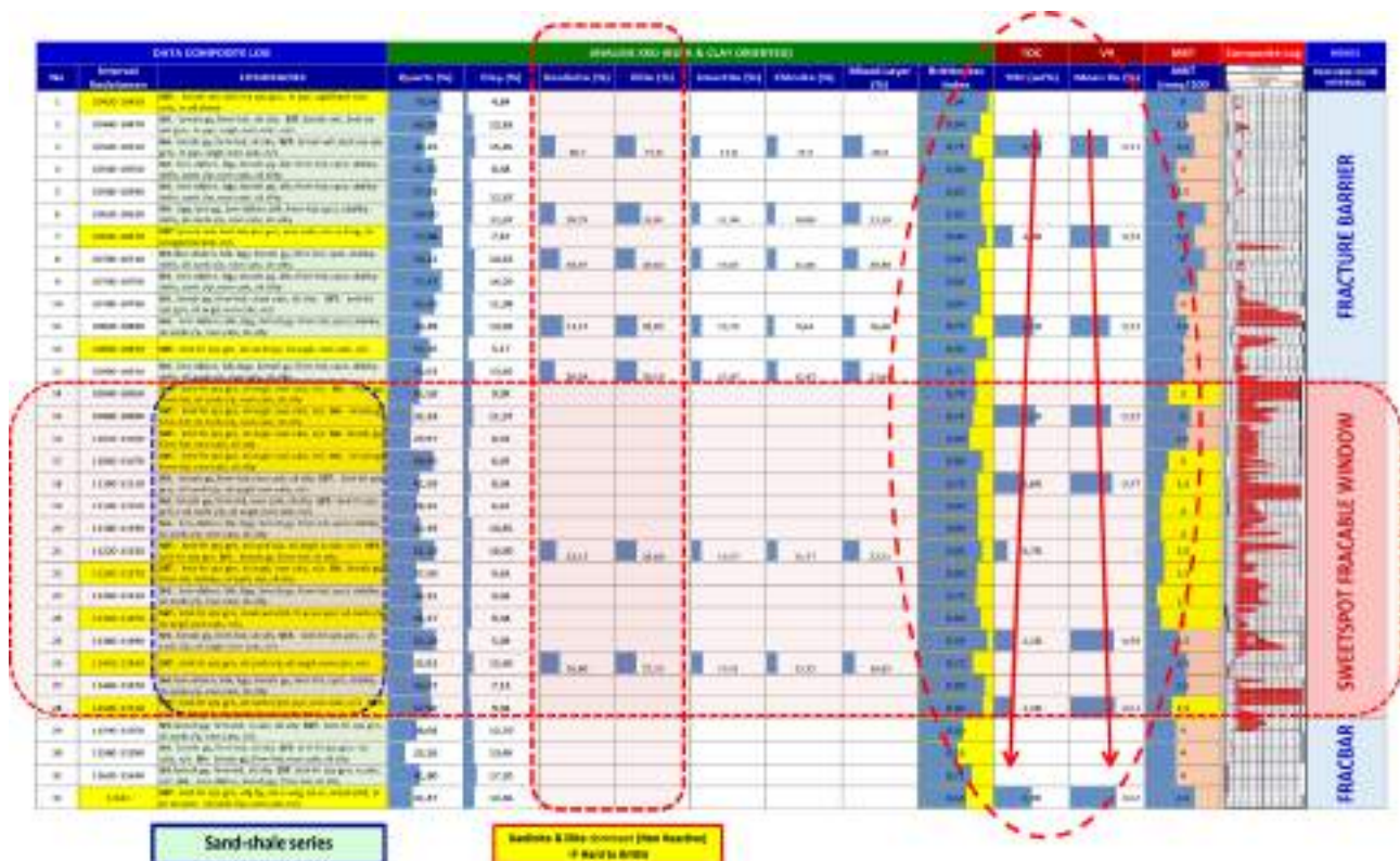
Figure 6. Correlation of lithofacies with the results of XRD (Clay Oriented) analysis, MBT, TOC, Ro from drill cuttings, and total gas from the composite log data.
