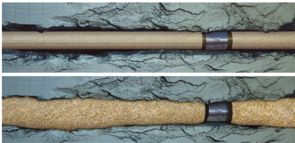
Figure 4: Shape Memory Polymer (SMP) pre and post activation that fill up wellbore gap.
