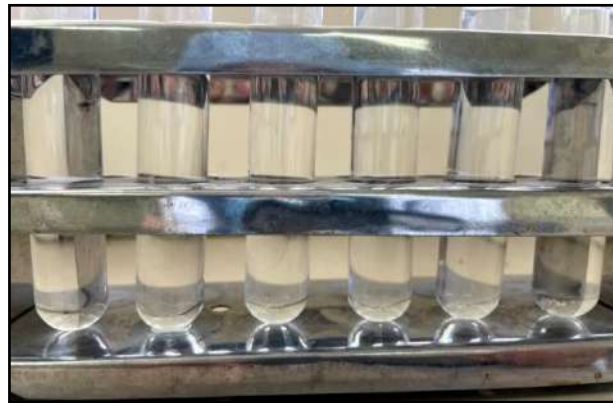
Figure 10. The Result of Polymer Aqueous Stability Test for Seventh-day at 60°C
