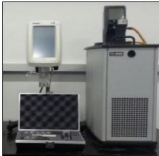
**Gambar 6. 10. Brookfield viscometer.**
