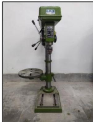
**Gambar 4. 7. Bench Drilling Machine**
