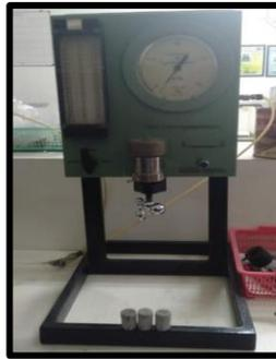
**Gambar 4. 15. Gas Permeameter**
