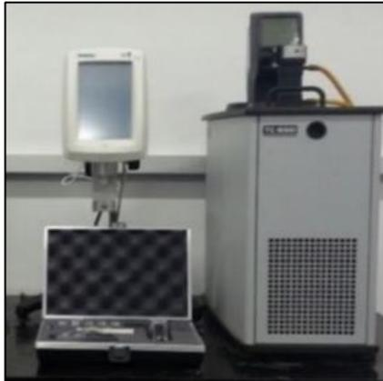
**Gambar 6. 10. Brookfield viscometer.**
