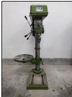
**Gambar 4. 7. Bench Drilling Machine**
