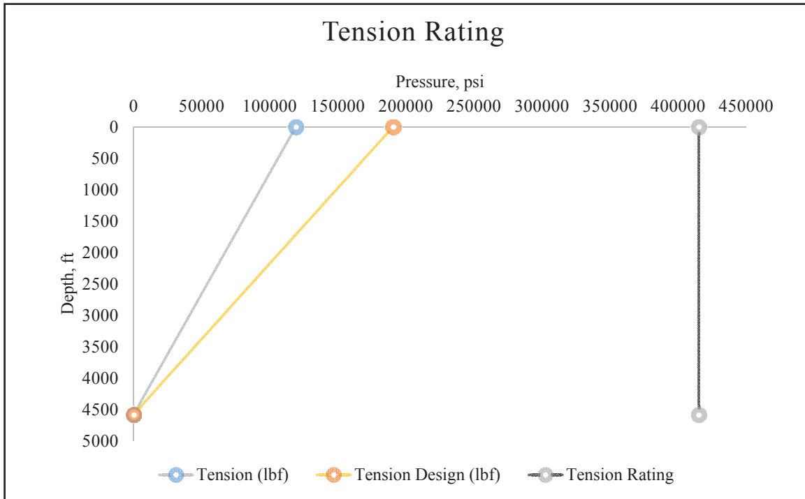
Figure 14 Tension rating of production casing.
