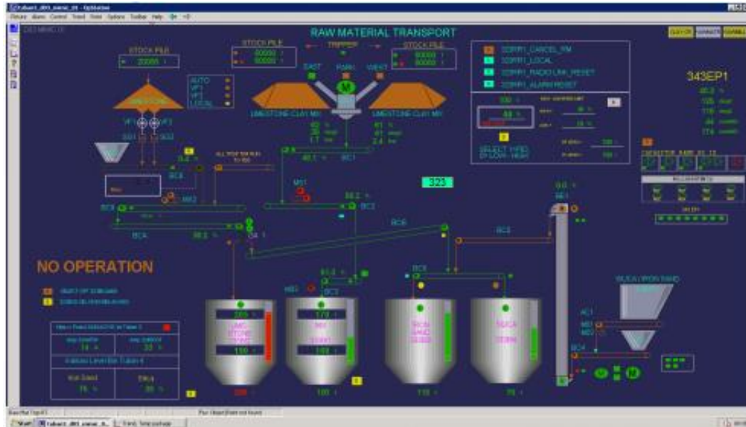
Gambar 1. PFD Raw Material Transport (sumber : CCR PT. Semen Indonesia, 2021)
