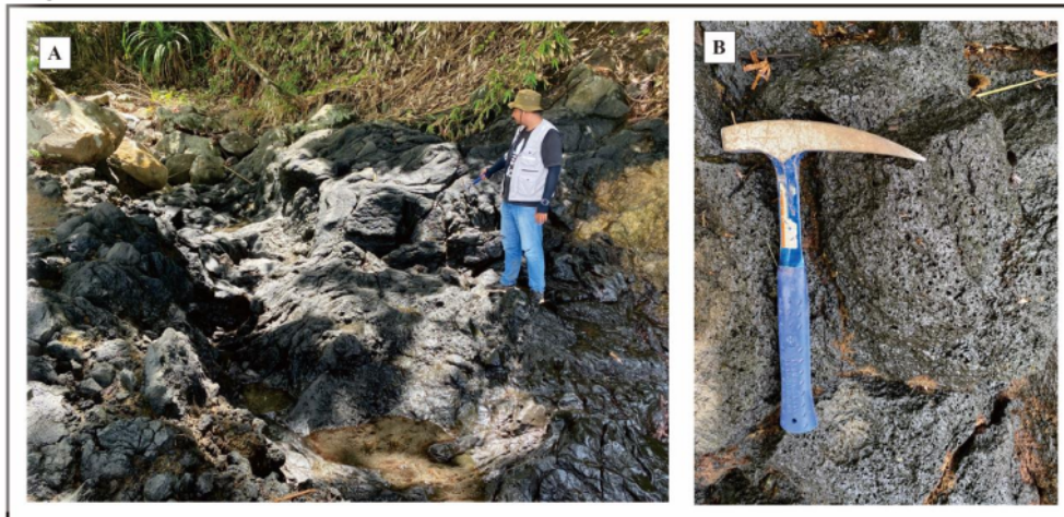
Figure 3. Idamdehe basalt lava outcrop shows the autobreccia structure of Arugasi
