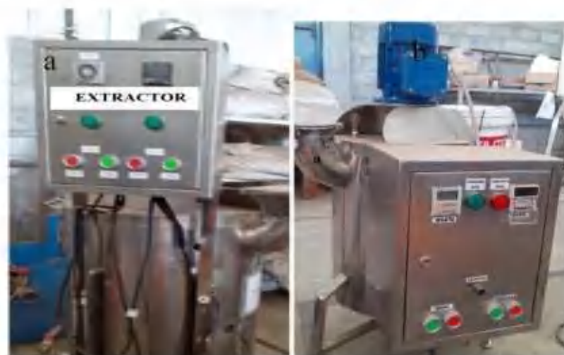
Figure 3. The equipment of Al-Alg catalyst formation (a) Extractor and (b) Reactor
