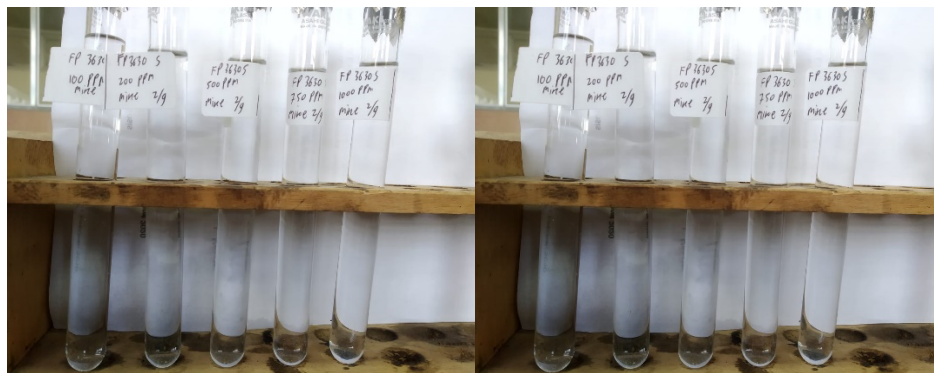
Figure 3. Aqueous Stability Result for Seventh-day at 25°C
