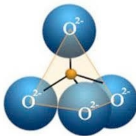
Fig 1. Tetrahedral silica structure
