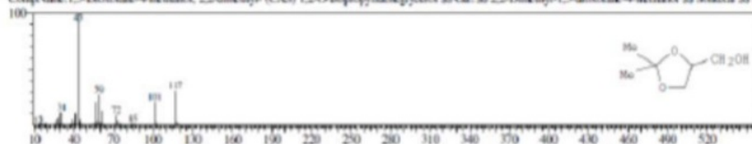
Supplementary 3. The results of GC-MS analysis in the reaction of Acetone and Glycerol using Al-Alg as catalyst at the temperature of 63°C during for four hours with the ration between the acetone mole and the Glycerol = 2:1 (mol/mol).
