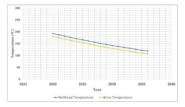
Figure 4. Wellhead and brine temperature drop vs year
