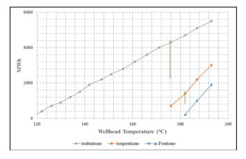
Figure 5. Electric power generated by each working fluid
