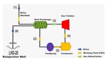
Figure 3. Binary cycle system power plant project
