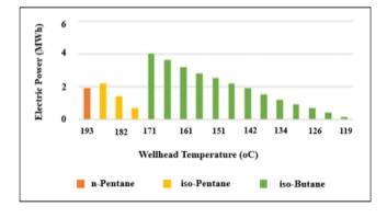
Figure 6. Wellhead temperature sensitivity for each working fluid
