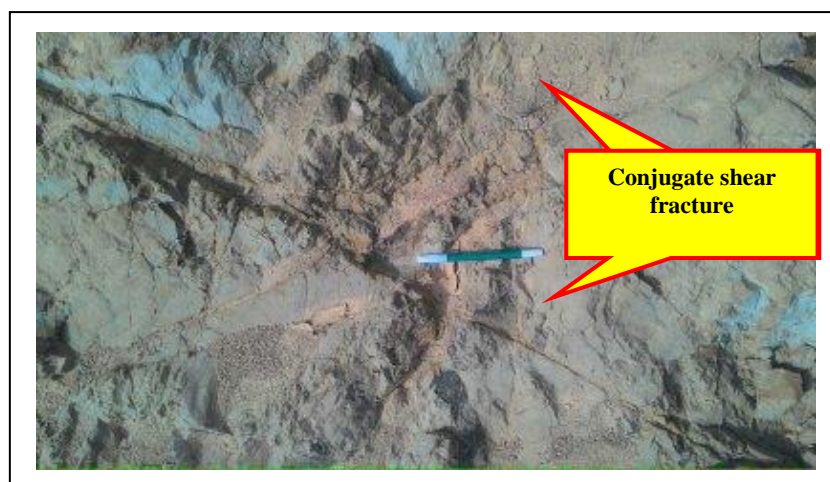
Fig. 7 Systematic shear joint on Nanggulan Formation that can be used to determine the direction of the maximum stress.
