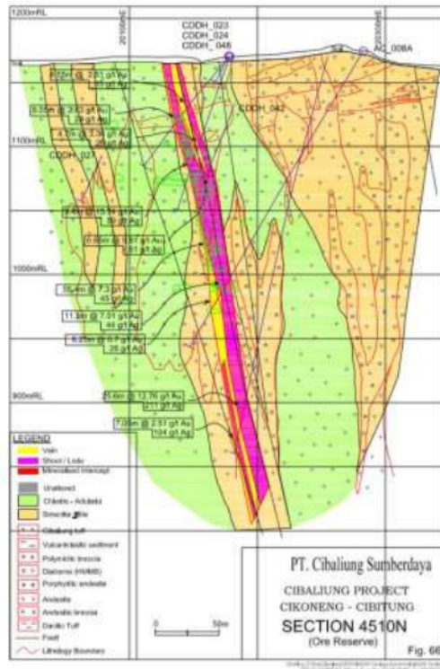
FIGURE 5. Section N4510 Cibitung Block (PT CSD)
