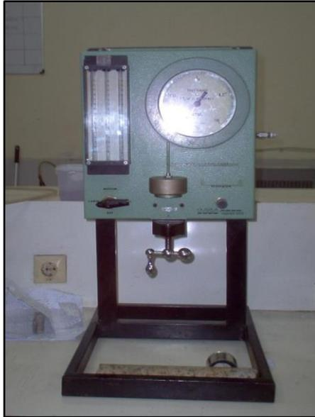
**Gambar 3.12. Gas Permeameter**
