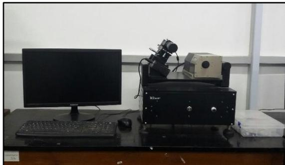
**Gambar 3.13. Rangkaian Alat *Spinning Drop Tensiometer***
