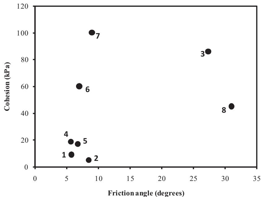
Fig.6. Shear strength of the filled discontinuities (Modified from Hoek & Bray, 1981)
