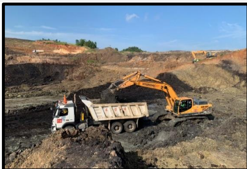
Gambar D.5 Loading Overburden
