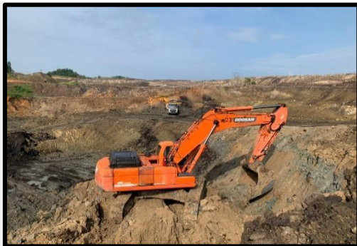
Gambar D.3 Pengupasan Overburden
