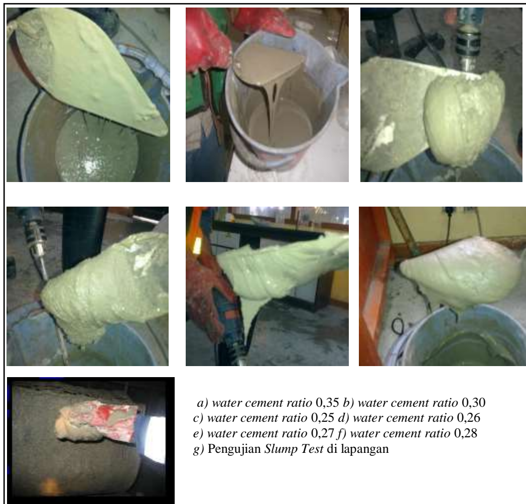
Gambar 6. Slump test
