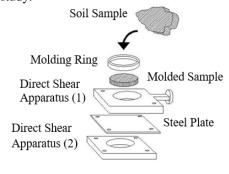
Fig 2. Illustration of adhesivity test
