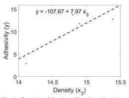
Fig. 9. Graphic of density effect for adhesivity value
