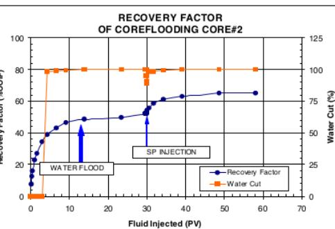
Gambar 9. Kadar air coreflooding test-2
