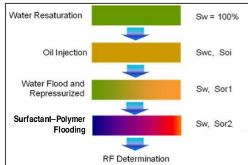
**Gambar 2.** Mekanisme *coreflooding test* di laboratorium (After Lemigas, 2012)
