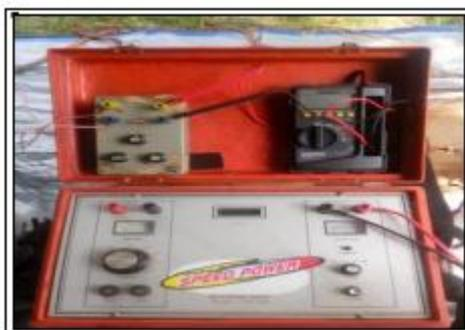
Gambar 2. Alat Resistivitymeter merek Naniura model NRD-300.
