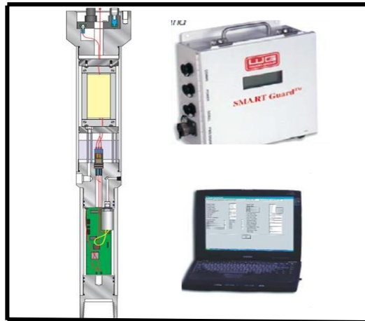
Gambar 3.8. Pressure Sensing Instrument (Cosco catalogue, 2009)
