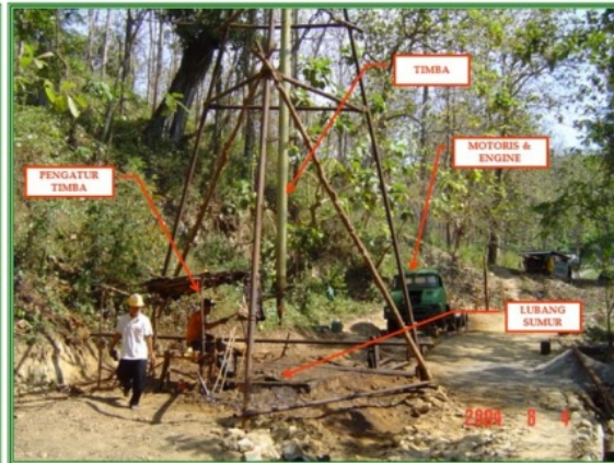
Figure 1. The Old Well Traditional Production Technology in the Banyubang field
