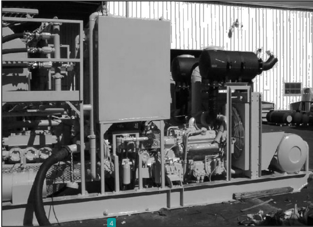
Gambar 7.3. Skit mounted cementing unit
