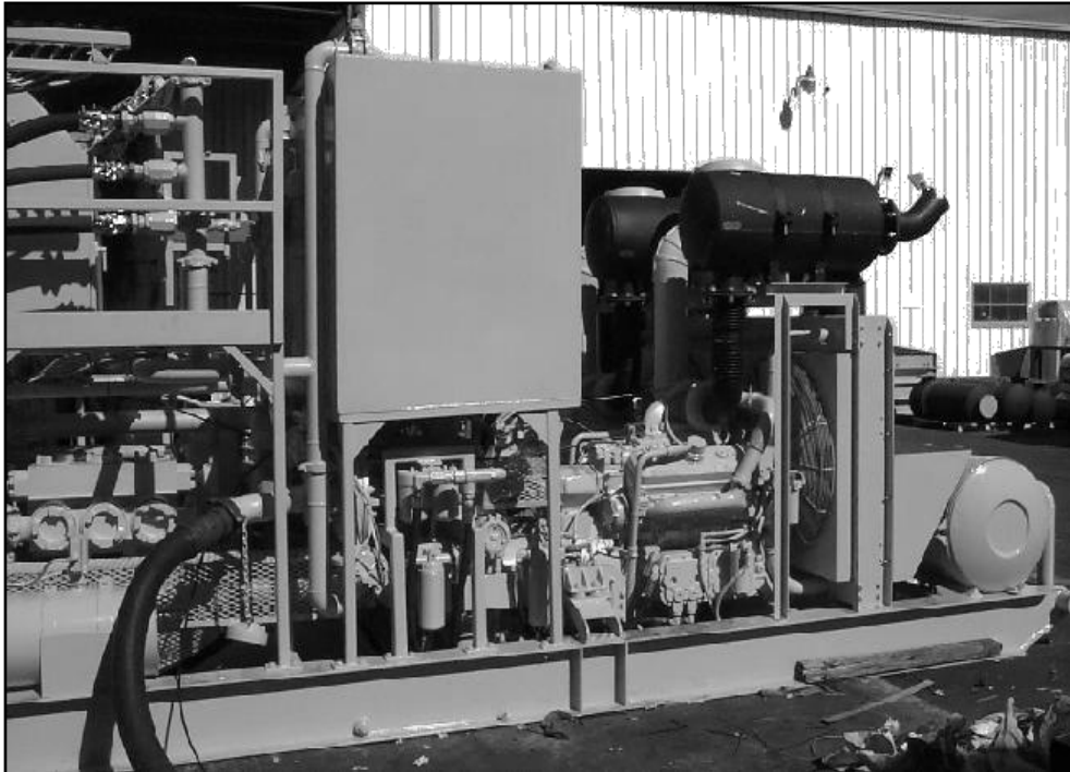
Gambar 7.3. Skit mounted cementing unit
