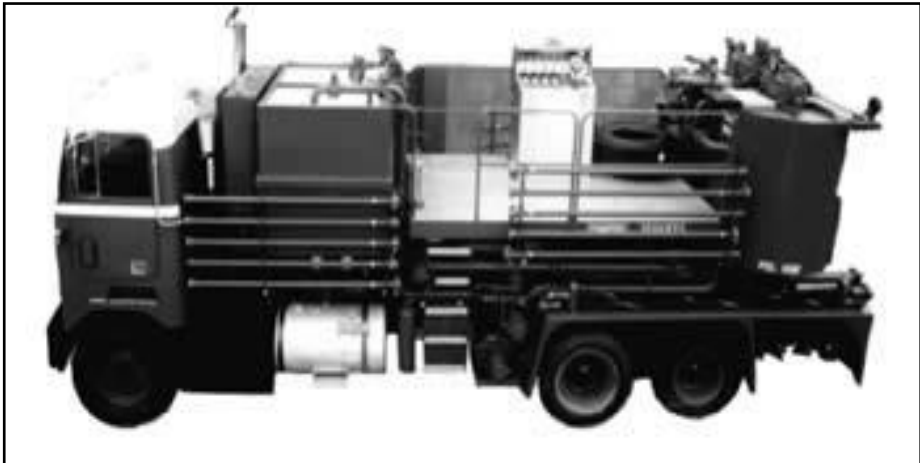
Gambar 7.1. Truck mounted cementing unit
