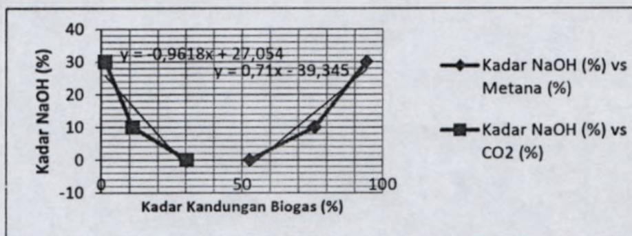
**Gambar 8.5. Kadar Kandungan Biogas vs Persentase NaOH**
