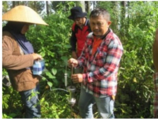
Figure 4. Measurement of mercury in soil by using Hg-meter.
