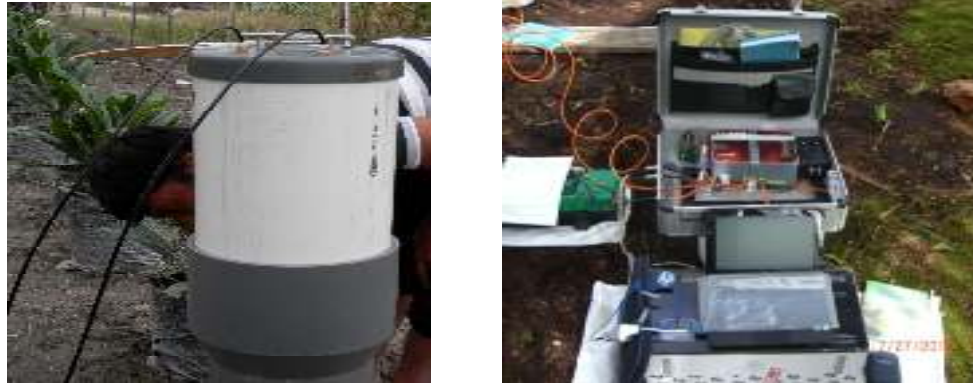
Figure 1 the CO 2 emission measurement methods using IRGA. Dark chamber (left), and IRGA equipment (right)
