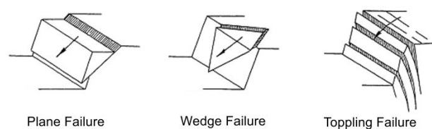
Figure 4. Types of rock slope failures: (a) block gliding (planar sliding), (b) wedge, (c) toppling [8].
