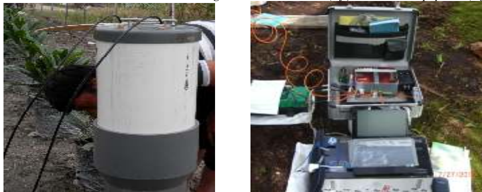
Figure 1 the CO 2 emission measurement methods using IRGA. Dark chamber (left), and IRGA equipment (right)
